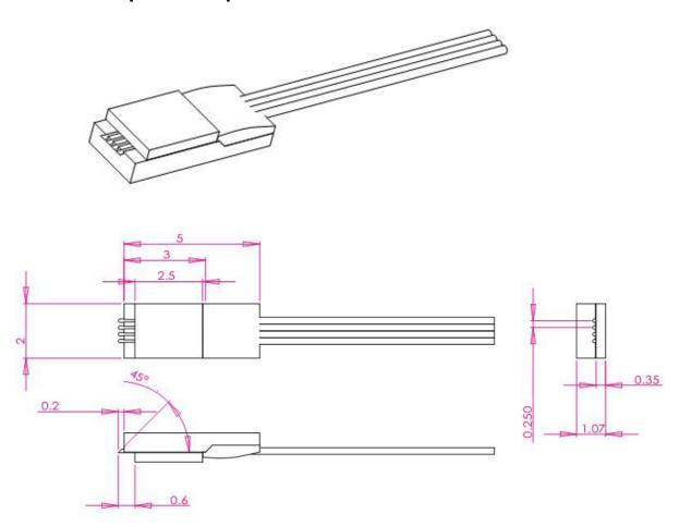
Optical Parameter: IL<0.8dB@1310nm for each channel.
